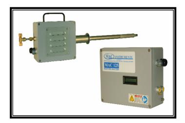
The MAC125-HT is a two piece solution for installations were the ambient temperature at the sample point exceeds 130°F / 55°C. The system consists of a probe that is inserted into the process and a remote electronics cabinet that can be mounted up to 100ft/30m away from the probe in an area where the ambient temperature is lower than at the sampling point. The MAC125-HT is **not** CE certified.
