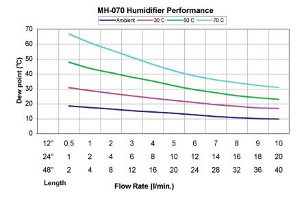
The above performance curves are for the MH-070. The MH-110 gives roughly a 3 degree higher outlet dew point than the MH-070. The MH-110 should be selected when a lower pressure drop is desired.
